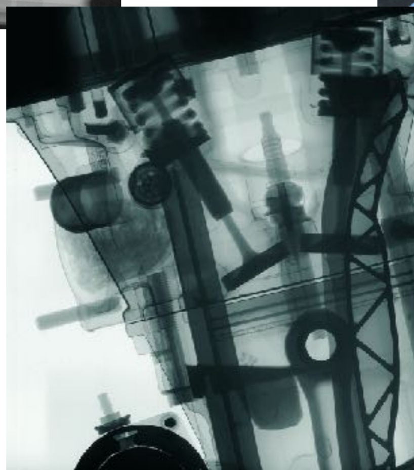
Neutron radiography of a motorcycle engine. FRM II/ANTARES
