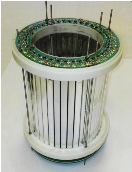
A view of strip assembly with SiPMs board
